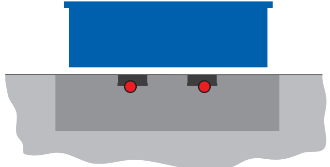
Cable installed directly into the floor
