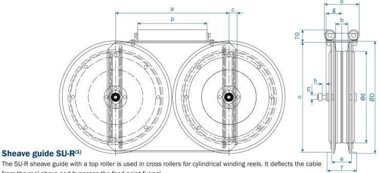
The SU-R sheave guide with a top roller is used in cross rollers for cylindrical winding reels. It deflects the cable from the reel above and bypasses the feed-point funnel.
